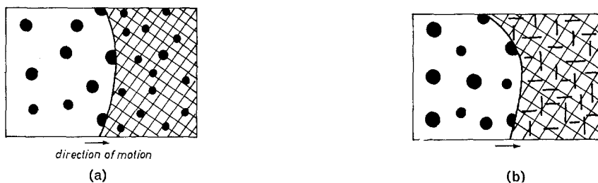
Figure 3 Schematic sketch of discontinuous recrystallisation. (a) The recrystallisation front sweeps out dislocations and sub-boundaries. (b) The recrystallisation front sweeps out dislocations and sub-boundaries and also transforms \theta' to \theta .
